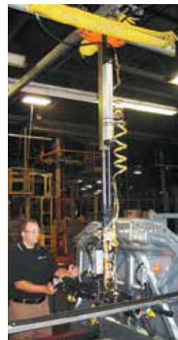
Torque tube with integrated vacuum handling device
